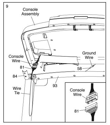
Set the console assembly on the Right and Left Handrails (84, 85). Make sure that no wires are pinched. Insert the excess Upright Wire (81) into the Right Upright (90).
